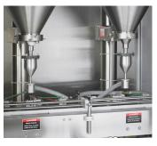
AUTOMATIC FEED FORWARD FEEDBACK: Automatic container tare weight/final weight calculations ensure an accurate fill. Feedback is automatically sent from the scale to the appropriate filling head to adjust auger revolutions for the next fill.
